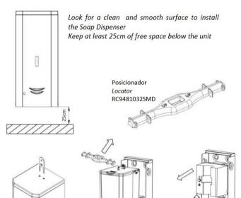
Open the unit with the provided key Remove the soap tank locator and the soap tank with the valve Remove the mechanism
